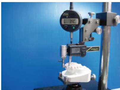
Figure 5. Transfer of torque and angulation to the BPD.
